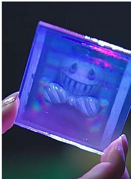
Denisyuk Hologram observed by transmission via halogen spot, after bleach but before drying.
